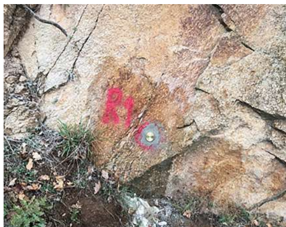
Figure 4: Stabilization of the basic leveling points R_1 (left) and R_3 (right).
