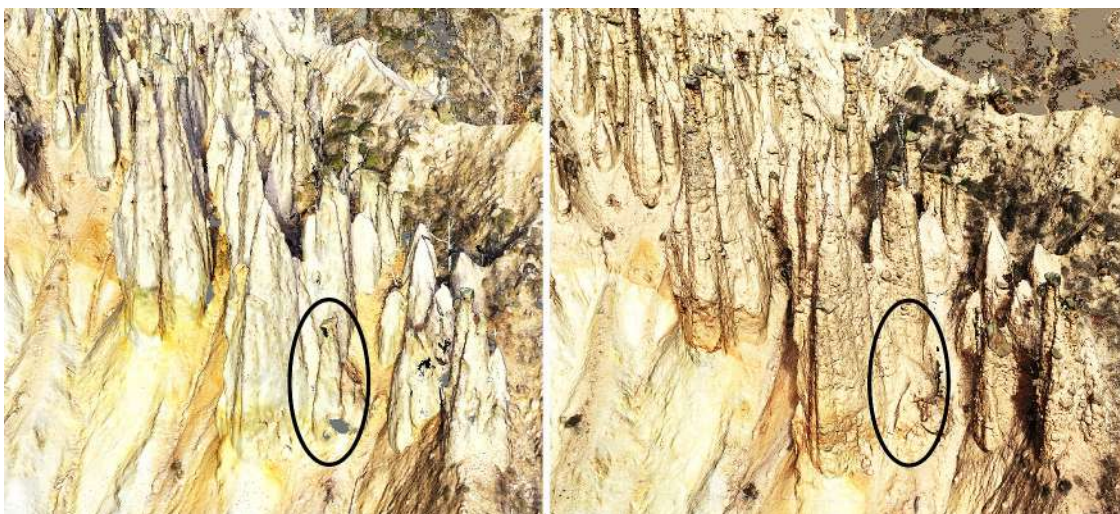
Figure 3: Difference in the level of detail between the 3D model reconstructed with automated flight plan made in 2018 year (left) and manual free-flight plan made in 2024 year (right) and identification of collapsed earth pillar marked with black ellipse on both images
