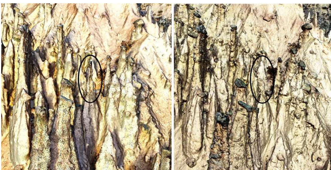
Figure 4: Identification of earth pillar with a lost cap made of rock between 3D model generated from 2018 mission (left) and model generated from 2024 mission (right)
